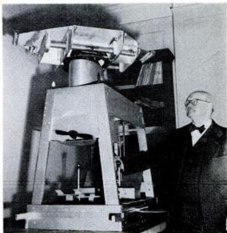
Mockup of convertiplane in Herrick's office is equipped with complete controls, revolving rotor head and forward propeller
